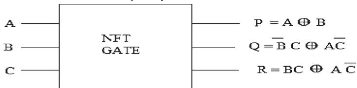
Figure 7: Block diagram of NFT GATE
