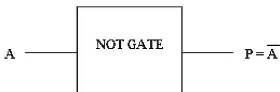
Figure 1: Block diagram of the NOT GATE
