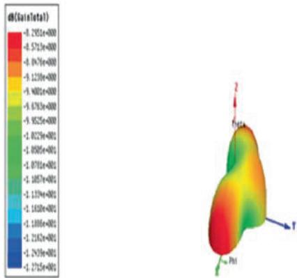
Fig-9 Gain at frequency 3.35 GHz
