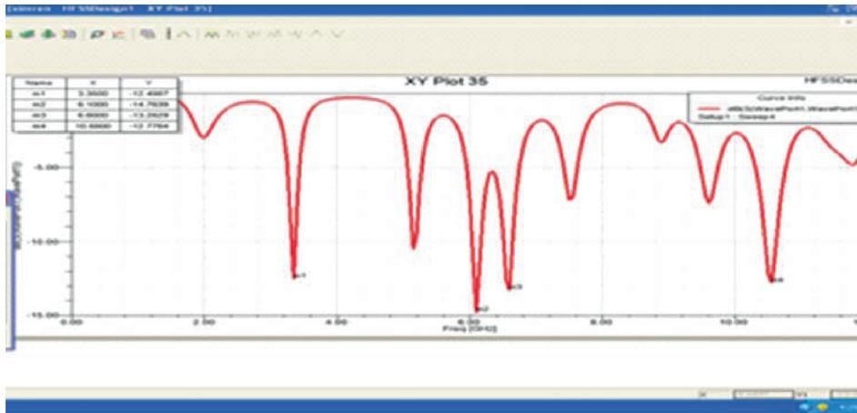
Fig 7-Return loss of unslotted octagon patch microstrip antenna VSWR 1.16 at frequency 3.35GHz , 1.44 at frequency 6.10GHz,1.55 at frequency 6.10GHz and 1.59 at frequency 10.55 GHz.
