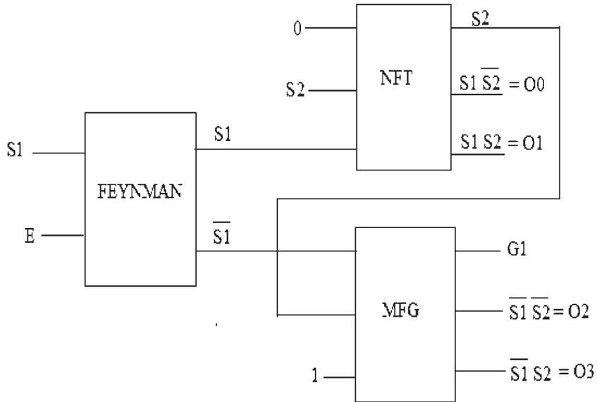
Figure 13 : Block diagram of the 2:4 reversible decoder with FG,NFT and MFG gates
