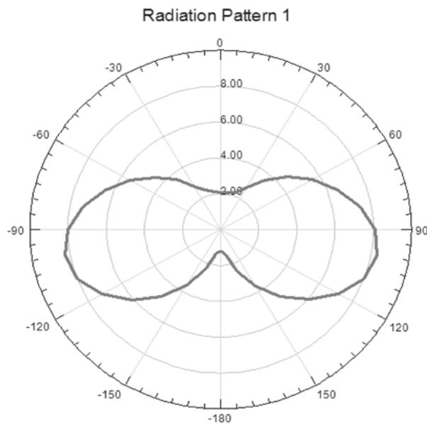
Figure 5: Radiation Pattern at 4.20 GHz
