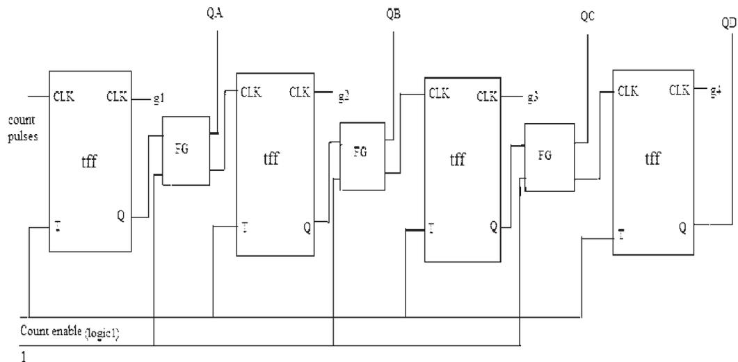
Fig. 4: block diagram of reversible asynchronous up counter
