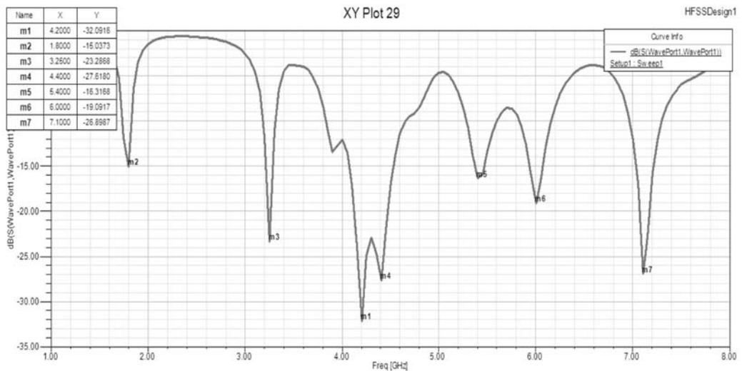
Figure 3: Return Losses or S-Parameter
