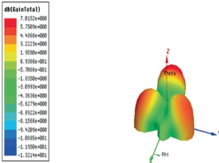
Fig 6-Gain at frequency 10.34 Ghz
