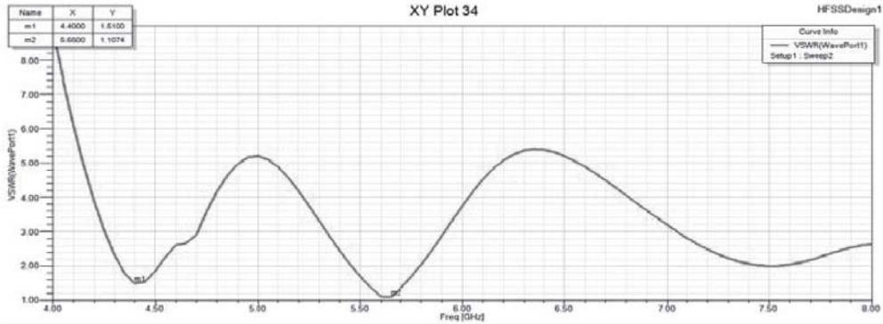
Fig.3 VSWR are on 4.4 and 5.65 GHz using FR4
