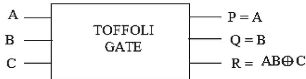
Figure 3: Block diagram of the TOFFOLI GATE
