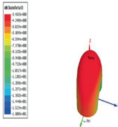
Fig-12 Gain at frequency 10.55 GHz
