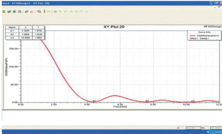
Fig 3- VSWR of slotted octagon patch antenna
