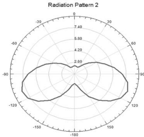
Figure 6: Radiation Pattern at 4.40 GHz
