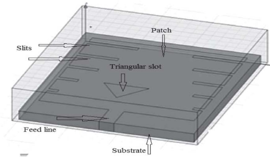
Figure 2: Isometric view of the multiband microstrip antenna
