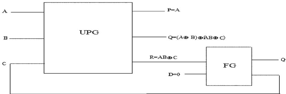
Fig 4: Block diagram of reversible triggered flip-flop
