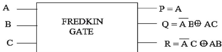
Figure 4: Block diagram of FREDKIN GATE
