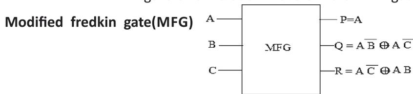
Figure 10: Block diagram of MFG gate
