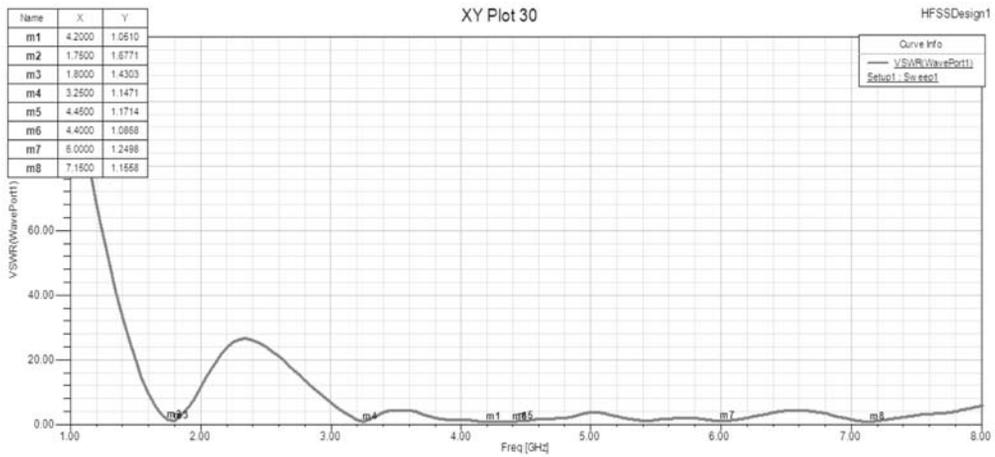
Figure 4: VSWR of Multiband Microstrip Antenna
