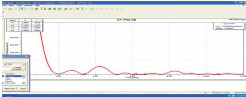
Fig - 8 VSWR of unslotted octagon patch microstrip antenna
