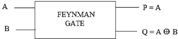
Figure 2: Block diagram of the FEYNMAN GATE
